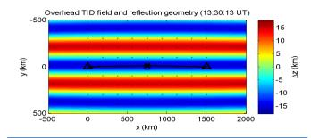
layer height: 280 km (untilted) period: 80 minutes horizontal wavelength: 400 km azimuth angle: -90 deg (wrt tx bearing) amplitude of height perturbation: 15 km
